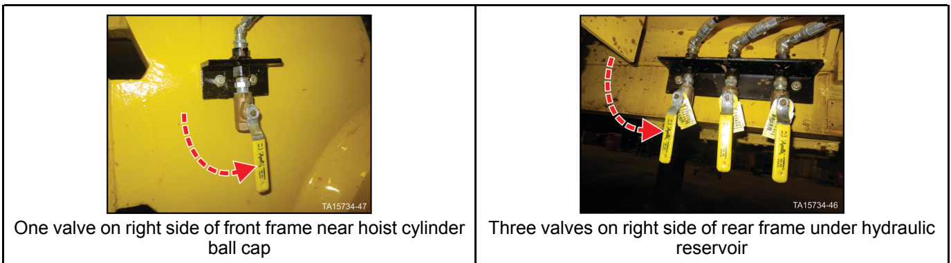
Figure 70: Open air reservoir bleed valves
