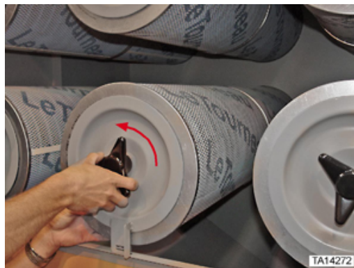
Figure 97: Removal of “KLENZ™” filter tabbed cover
