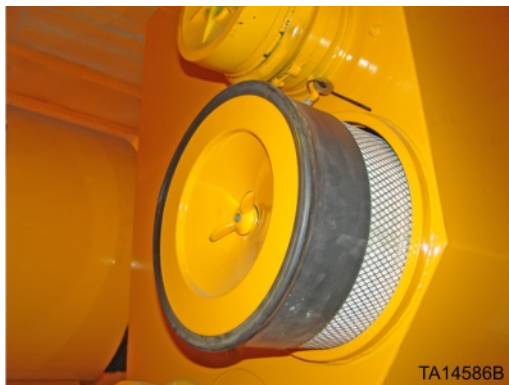
Figure 116: Install outer filter element
