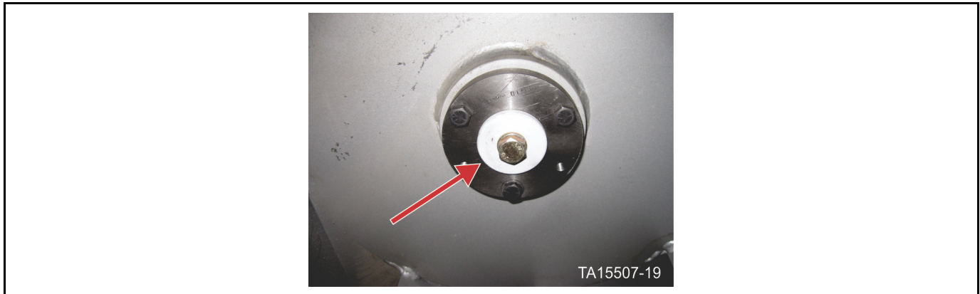
Figure 56: Blower wheel bushing capture bolt
