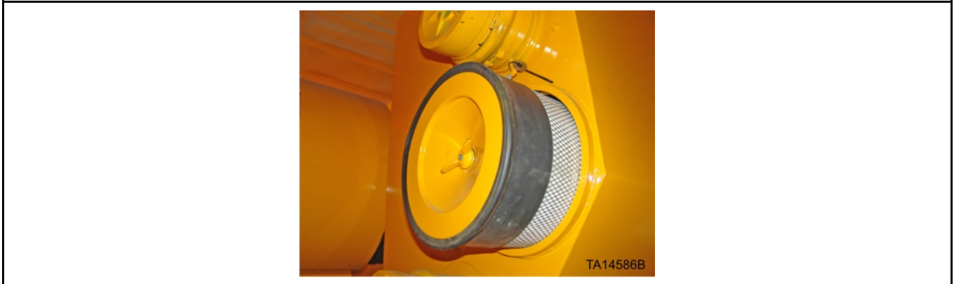
Figure 109: Engine safety outer filter rubber sleeve
