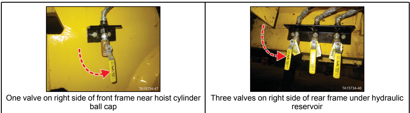
Figure 93: Open air reservoir bleed valves
