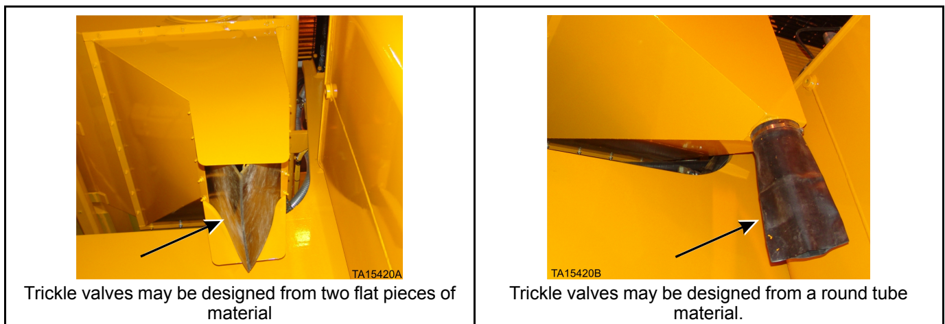
Figure 10: Trickle valve designs
