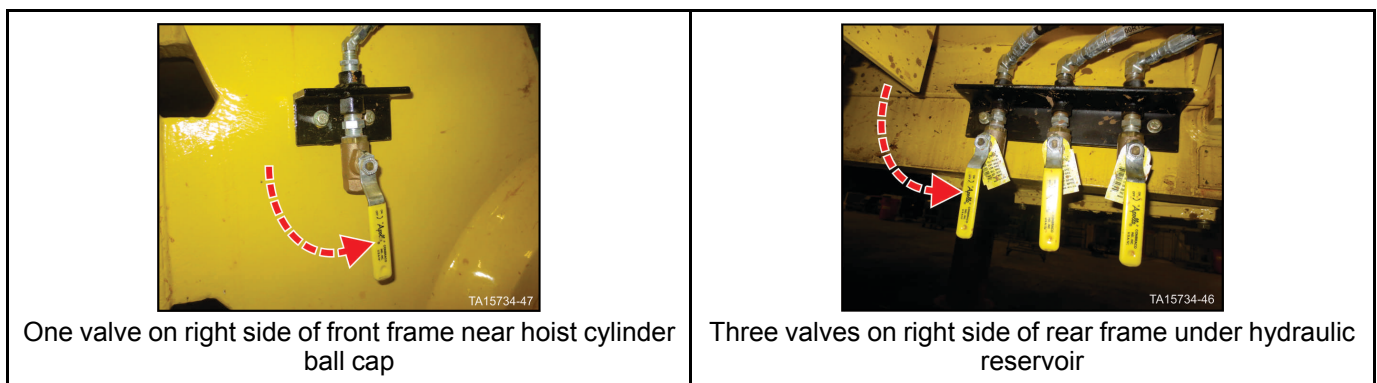
Figure 44: Open air reservoir bleed valves
