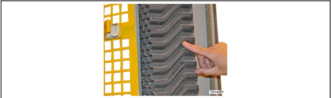
Figure 80: Proper position of mist eliminator baffles
