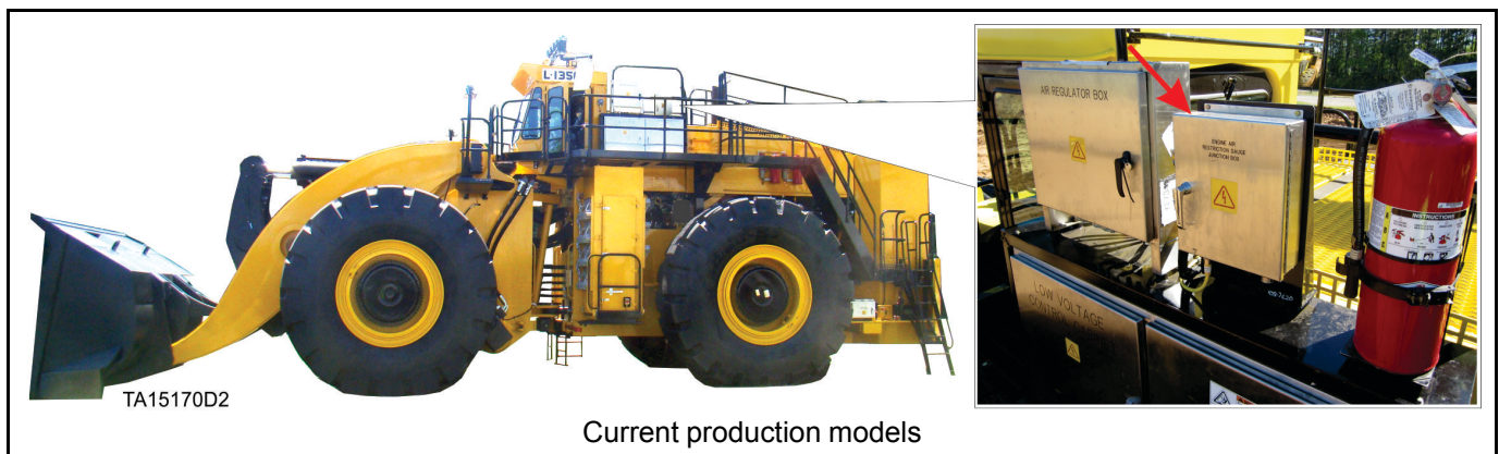
Figure 120: Engine filter restriction gauge location (current location)
