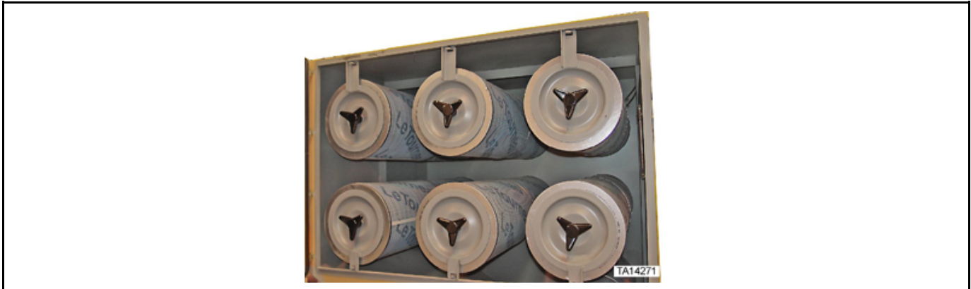
Figure 85: View inside typical filter chambers (number of filters might vary by machine model)
