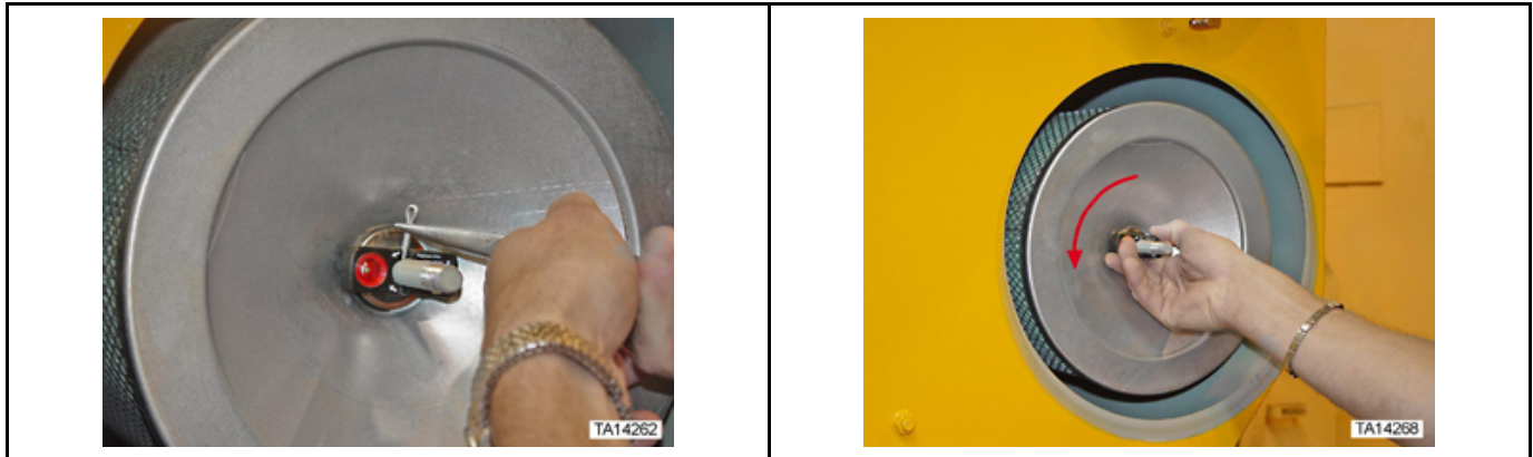
Figure 111: Removal of cotter pin from engine secondary (safety) filter indicator wing nut and Removal of engine secondary (safety) filter indicator wing nut
